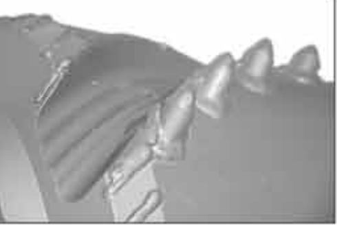
Heavy-duty carbide hard surfacing along the body of the reamer helps protect against abrasive ground and extend the life of the reamer. Carbide cutters placed along the body of the reamer, delivering superior cutting power.
