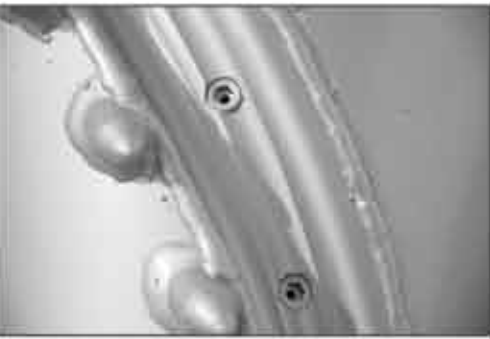
Heavy-duty carbide hard surfacing along the body of the reamer helps protect against abrasive ground and extend the life of the reamer. Carbide cutters placed along the body of the reamer, delivering superior cutting power.
